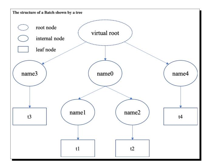
"Hierarchical named tensors" refers to a set of tensors where their names form a hierarchy. Suppose there are four tensors [t1, t2, t3, t4] with names [name1, name2, name3, name4], where name1 and name2 belong to the same namespace name0, then the full name of tensor t1 is name0.name1. That is, the hierarchy lies in the names of tensors.
