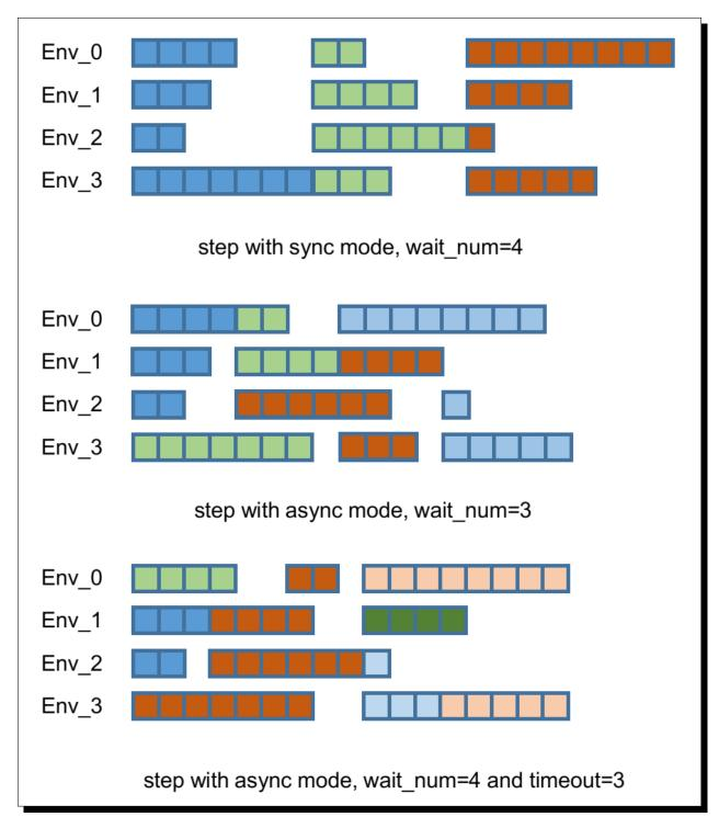
By default, parallel environment simulation is synchronous: a step is done after all environments have finished a step. Synchronous simulation works well if each step of environments costs roughly the same time.
