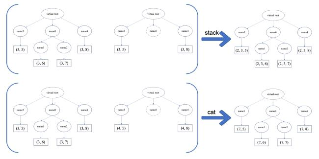
We only consider the heterogeneity in the structure of Batch objects. The aggregation operators are eventually done by NumPy/PyTorch operators (np.stack, np.concatenate, torch.stack, torch.cat). Heterogeneity
